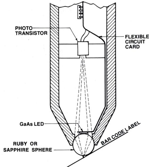
Schematic of Intermec's RUBY WAND Scanner
