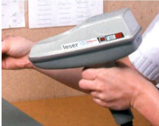
The pilot scanners worked well as long as no one dropped them. Unfortunately, when dropped the fragile component used to mount the scanning mirror broke, rendering the scanner inoperable. This problem delayed the production rollout while limit stops were incorporated into the design. Subsequently, the 1600 became a good product with many units sold.
