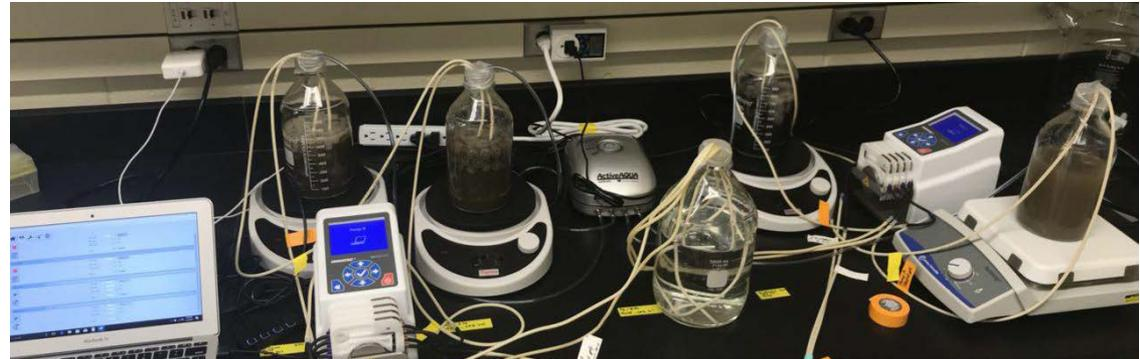
Moving bed biofilm reactors to study different carriers for nitrogen removal in biofilm
