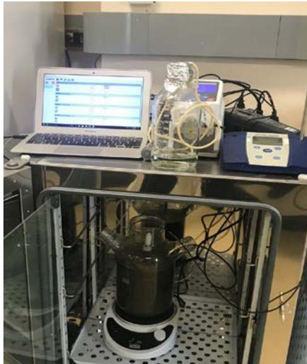
Bioreactor with intermittent aeration to study nitrogen removal via short-cut nitrification/denitrification
