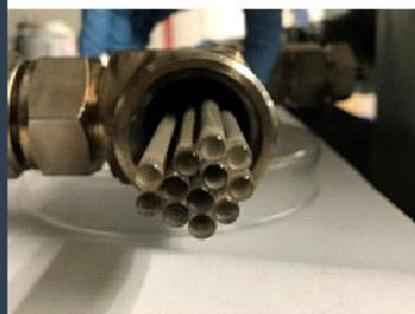
Waveguides with Catalyst
