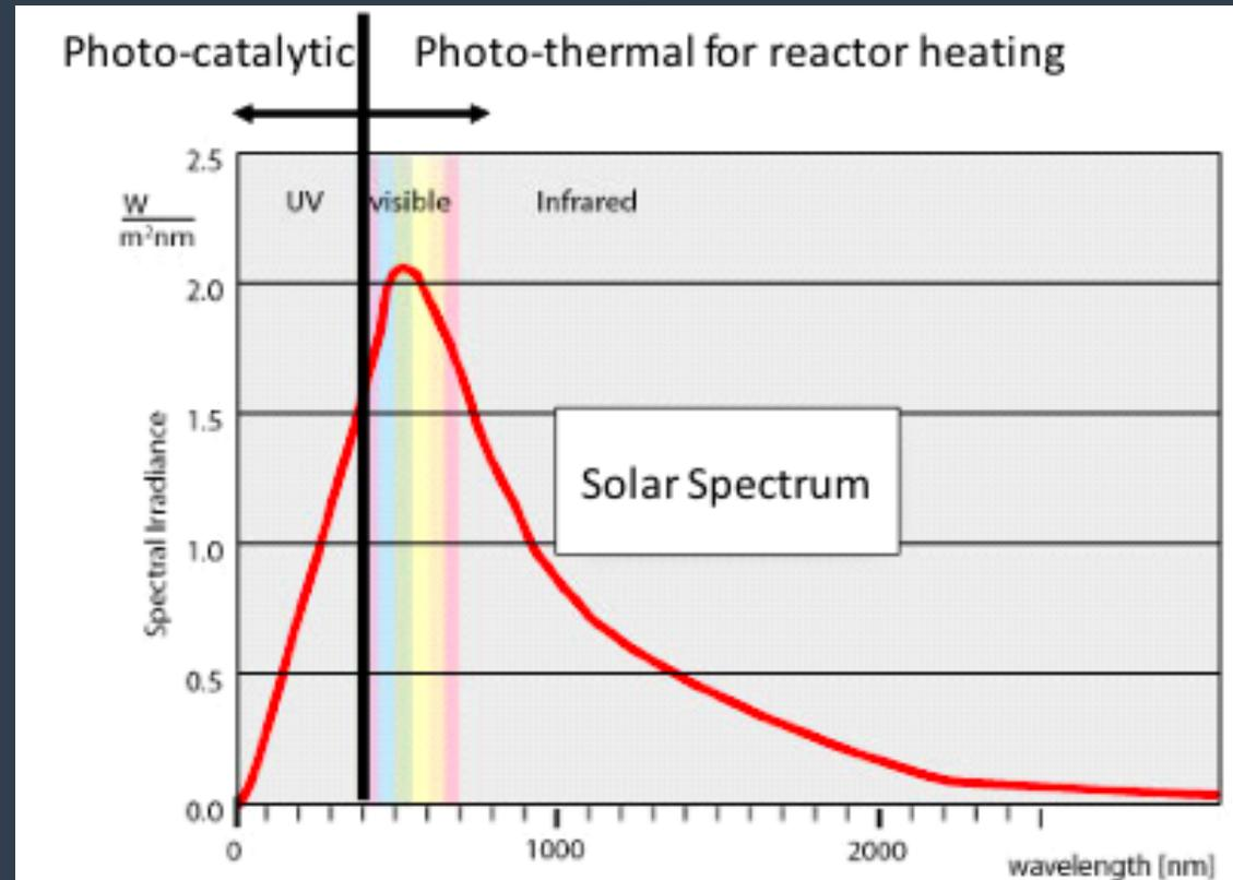
**Figure Y: Solar Spectrum.** A method we intend to use to reduce the reactor heating load is to take advantage of the entire solar spectrum to provide photocatalytic energy to drive the reaction and photothermal energy to heat the reactor.
