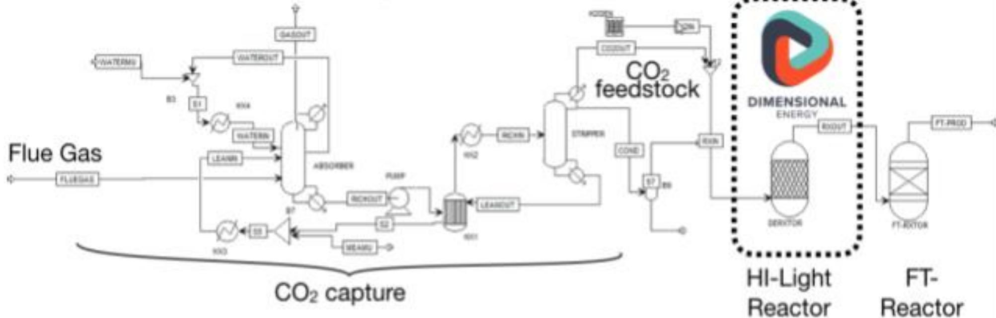
**Figure 1.4** Schematic illustration of the 'CO<sub>2</sub> refinery'. The HI-Light reactor developed at Dimensional Energy is integrated with upstream CO<sub>2</sub> capture and downstream syngas conversion in a Fischer-Tropsch (FT) reactor to form higher hydrocarbon products.
